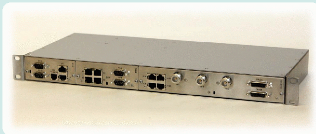
Protection Switching Unit
